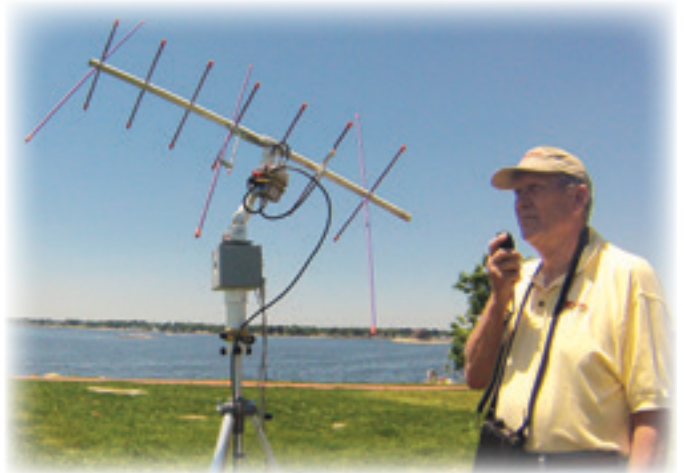
The WRAPS az-el rotator system mounts on a camera tripod. [Photo courtesy Mark Spencer, WA8SME]
